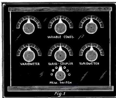
The Completed Instrument with Its Various Condenser and Variometer Handles Symmetrically Arranged.
