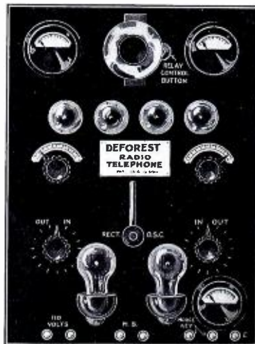
The New Radio Telephone Set Which Operates from Your 110-Volt A. C. Supply.
